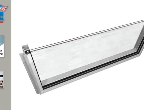
The Series 8100 Fixed Window has a 4-1/2" (114 mm) deep frame designed to match typical building conditions, including our entrances and storefronts. An efficient thermally insulated frame accepts 1" (25 mm) glazing. Available in an array of architectural coatings and anodized finishes.
